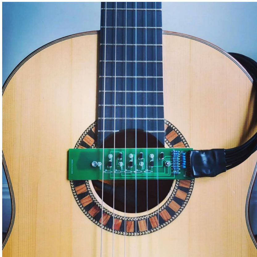
Figure 27 Custom light sensor for Cryptoguitar
